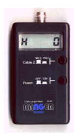
For use with RG59 (75 $\Omega$ ) and RG58 (50 $\Omega$ ) or equivalent coaxial cable, this meter provides a direct readout in metres of the length of an unterminated run of coaxial cable with a resolution of 2-3 metres. A single range of 2.5 to 400 metres on a 4 digit LCD display is provided with automatic indication of open circuit and short circuit conductors. By this means, the location of a short circuit or open circuit in cable runs of up to 800 metres may be found.
