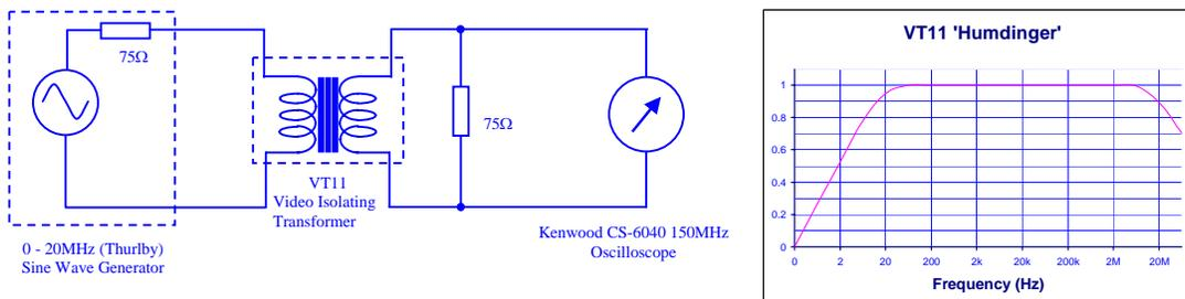
Fig 1 VT11 'Humdinger' Video Isolating Transformer Test Circuit and response curve
